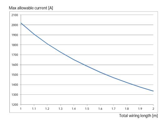
It is very important to stay within these limits, as exceeding them will likely damage the welder. For continued protection, the *kWeld* system allows you do dial in your system cabling length, and it calculates an appropriate current limit from that using the above formulas. When not using the standard cabling configuration, it is strongly recommended to adjust this configuration accordingly.
