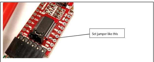
Make sure that the voltage switch on the adapter is **set to 3.3V** (it ships with the jumper installed in the wrong position).
