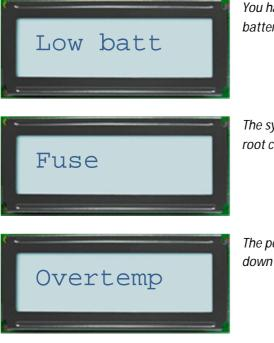
You have enabled a battery voltage warning level, and the battery voltage is lower than that.
