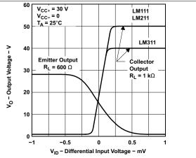
Figure 8. Voltage Transfer Characteristics and Test Circuits
