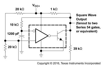
Figure 16. 100-kHz Free-Running Multivibrator
