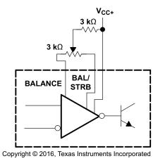
If offset balancing is not used, the BALANCE and BAL/STRB pins must be unconnected. It is also acceptable to short
