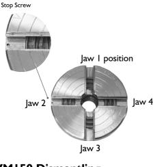
All the backing jaws are numbered to ensure easy assembly. The number two jaw is where the stop screw is as pictured on the left.
