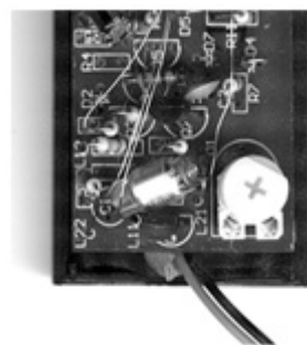
Figure 3. Internal Fine Adjustment Screw - with battery connected, and unit turned on to half-way, rotate adjustment screw until the unit just stops beeping. (See instructions).
