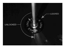
To unlock your lift, turn lift handle counterclockwise to the "UNLOCKED" position
