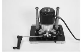
8. With the Mast-R-Lift<sup>™</sup> II Crank handle, retighten the tensioning cap screw. (Figure 7)
