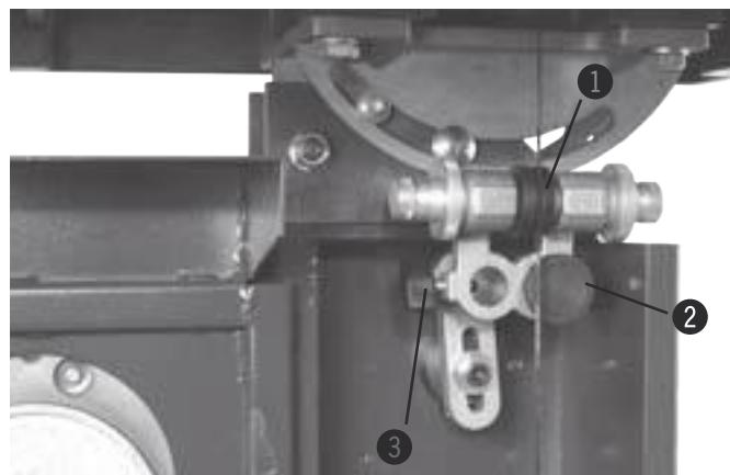
The side guide rollers should touch the saw blade slightly so as to obtain a straight and vibration-free cut.
