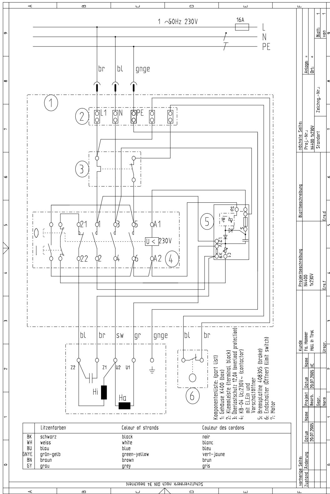
Fig. 22: Circuit diagram 1x 230 V
