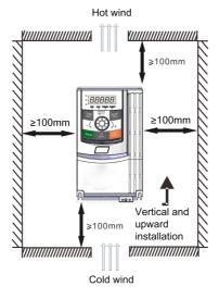
Fig.3-1 single one installation illustration
