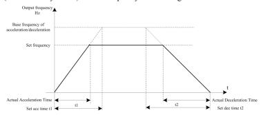
Fig.5-2 Illustration of acceleration/ deceleration time
