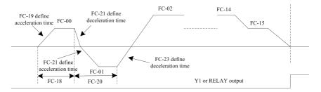
Fig.5-27 simple PLC illustration
