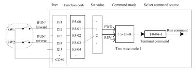
Fig.4-8 Illustration of terminal control start-stop mode
