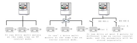
Fig.4-26 Switching of multi-group motors
