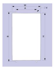
Tab.2-4 Wall-mounted mode installation dimensions of S1100V under 22KW
