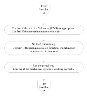
Fig.4-7 V/F control mode running steps
