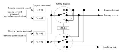
Fig.4-22 Illustration of motor running direction
