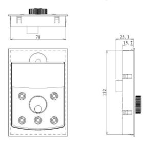
Fig.2-7 outer keyboard with plate installation dimension
