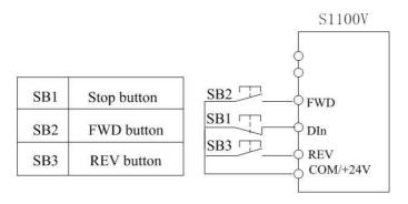
Fig.5-9 Three wire control mode 1
