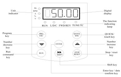
Fig.4-2 Schematic diagram of operation panel 2
