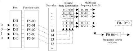
Fig.4-21 Illustration of multi-speed control mode
