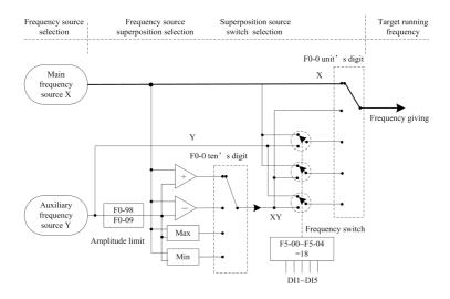
Fig. 5-1 Illustration of frequency source superposition
