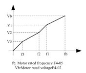
Fig.5-5 schematic diagram for V/F curve setup
