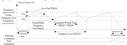
Fig.5-25 Swing Frequency Working Diagram
