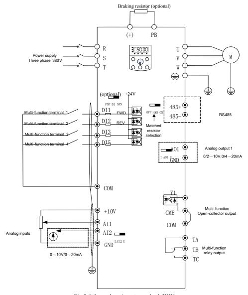
Fig.3-6 three-phase inverter under 1.5KW
