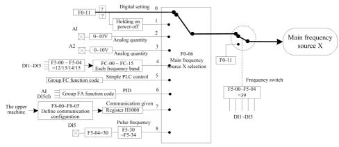
Fig.4-17 Illustration of main frequency source setting
