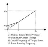
Fig.5-4 Illustration of Manual Torque Boost
