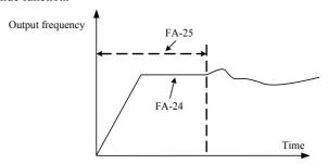
Fig.5-24 PID initial value function illustration
