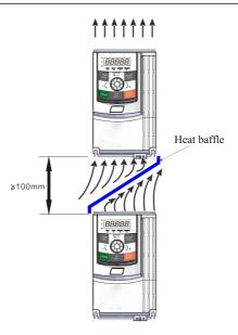
Fig.3-2 S1100V installation illustration
