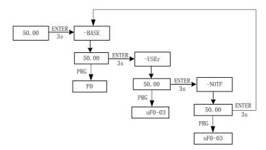
Fig.4-4 operation diagram of the menu mode switch
