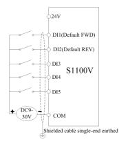
Fig 3-11 Four different wiring diagram
