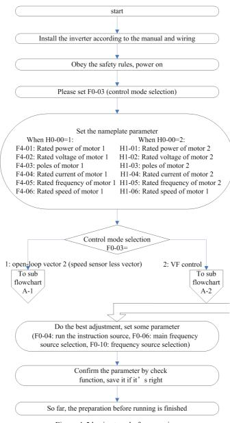
Figure 4-5 basic steps before running
