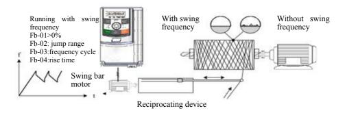
Fig.4-20 Illustration of swing frequency application setting
