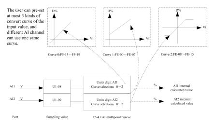
Fig.4-28 The actual given of AI signal
