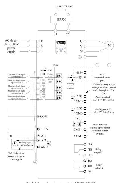
Fig.3-8 three-phase inverter within 37KW~55KW
