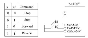
Fig.5-8 two wire control mode 2
