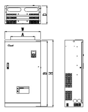
Fig2-7 Installation dimensions of metal mode above 160KW
