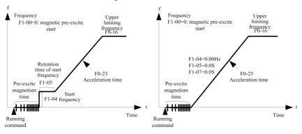
Fig.4-12 Pre-excited magnetism start illustration
