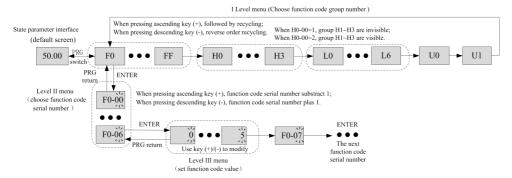
Fig.4-2 three-level menu operation flow chart
