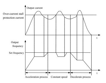
Fig.5-21 Over-current stall protection illustration
