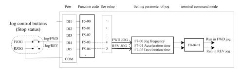
Fig.4-16 Parameter setting illustration of DI mode jog
