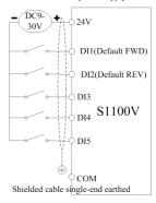
DI terminal connection Mode 4: DI dial switch in PNP mode and with external power supply
