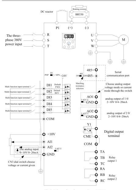
Fig.3-9 three-phase inverter above 75KW
