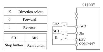
Fig.5-10 Three wire control mode 2
