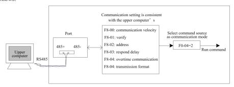
Fig.4-10 Illustration of communication control start-stop mode
