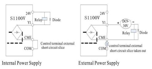
Fig.3-12 Schematic diagram for digital output terminal Y1 wiring
