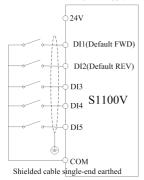
DI terminal connection Mode 3: DI dial switch in PNP mode and without external power supply
