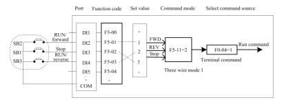
Fig.4-8 Illustration of terminal control start-stop mode
