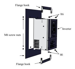
Fig.3-4 S1100V Wall-mounted installation instruction of sheet metal structure
