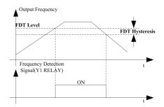
Fig.5-15 FDT electrical level illustration
