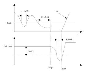
Fig.5-31 Sleep process frequency illustration
