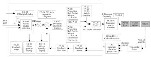
Fig.4-19 Illustration of frequency closed loop control
