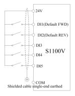
DI terminal connection Mode 2: DI dial switch in NPN mode and with external power supply
