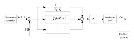
Fig.5-22 Process PID principle schematic diagram
