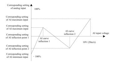
Fig.5-29 Multi-point corresponding illustration
