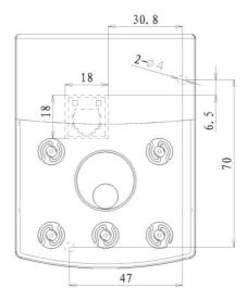
Fig.2-8 outer keyboard without plate installation dimension
