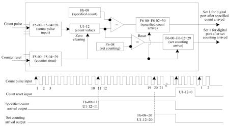
Fig.4-25 Counting mode function code setting
