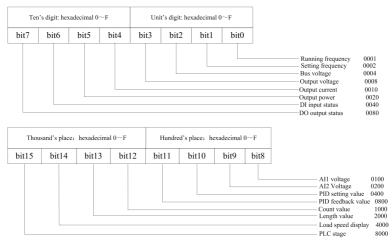
Fig.5-17 LED running display illustration
