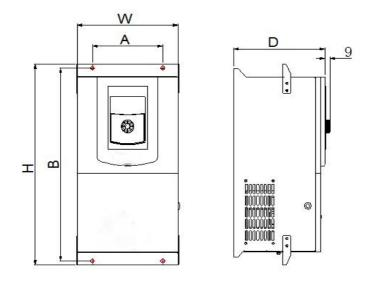
Fig2-5 Installation dimensions of metal mode within 11~37KW
