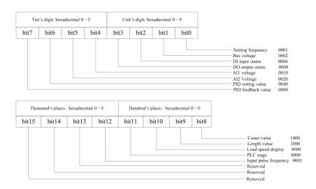
Fig.5-8 LED stop display illustration
