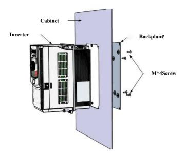
Fig.3-3 S1100V Wall-mounted installation instruction of plastic structure
