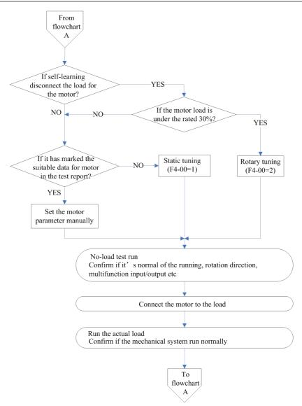
Fig.4-6 open-loop vector control running steps
