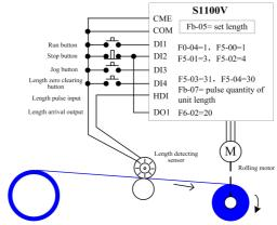
Fig. 4-24 Examples of fixed-length control function
